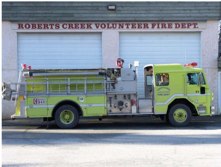
Engine 4 was built on a Peterbilt chassis by Anderson Engineering in 1991. It can carry up to 6 Firefighters to scene. In the reserve position it can operate as a pumper or in shuttle operations and carries 800 gallons supplying a 1050IGPM pump.
