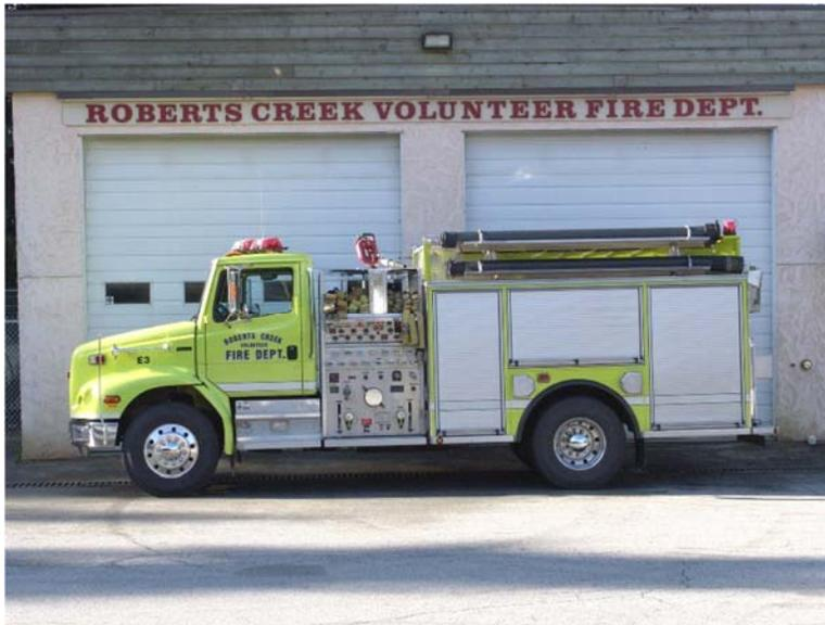
Engine 3 is built on a Freightliner FL112 chassis and was manufactured by Hub Fire Engines in 1999. It carries three fire fighters.
